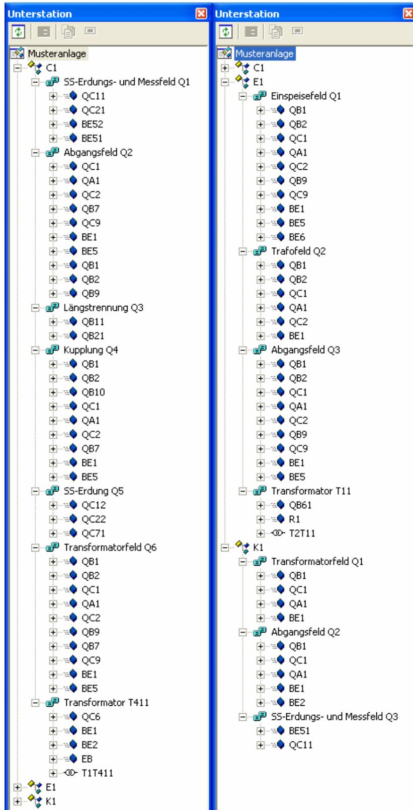
The SCL representation is hierarchical with substation, voltage and bay levels as shown in the left-hand picture. The pieces of equipment are clearly assigned to the bays.
